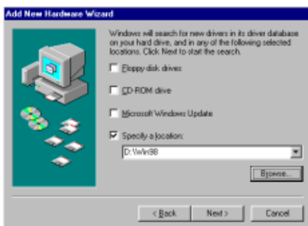
Figure 12: Select Specify a location. Insert the Motion CD into the CD-ROM drive. Browse to :\\MotionCD\\Windows\\MCAPI\\Current\\Win2000 or:\\MotionCD\\Windows\\MCAPI\\Current\\Win98. Select the *.inf file
