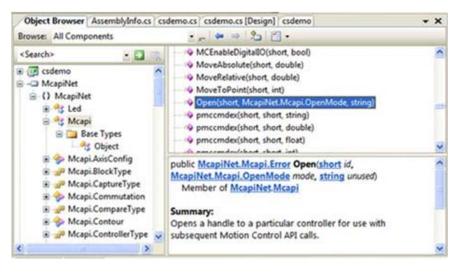
All the programming constants of the MCAPI function library have been migrated to .NET enumerations. McapiNet methods require the use of the correct enumeration types. This makes it almost impossible to pass a bad value for a constant to a McapiNet method in your program. The Open() method for instance will only except a Mcapi.OpenMode value for the open mode, Visual Studio will consider any other value a compile time error.
